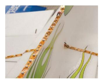
4 This strip running along the top edge of the fuselage will light up the canopy outline and give me a good reference point to keep the plane orientated in the air. This strip of lights could be ran completely around the plane but I kept them off the bottom just in case I cannot pull the plane out of the air during a hover and it has to land on its belly.
